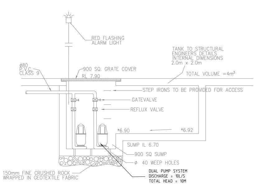
BASEMENT PUMPING SYSTEM SECTION A-A N.T.S.
